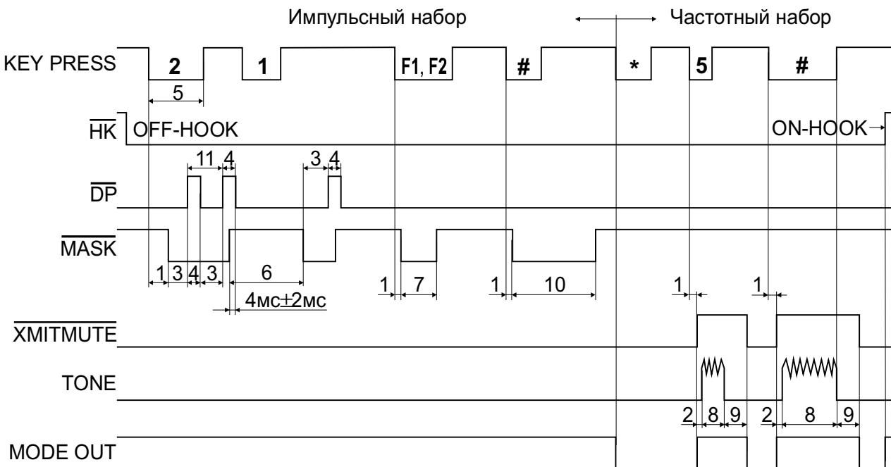
1 -  $t_d(\text{KEYL-MASKL})$ ,  $t_d(\text{KEYL-XMITMUTEN})$ . 2 -  $t_d(\text{XMITMUTEN-TONE})$ . 3 -  $t_w(\text{DPL})$ . 4 -  $t_w(\text{DPH})$ . 5 -  $t_w(\text{KEYL})$ .
